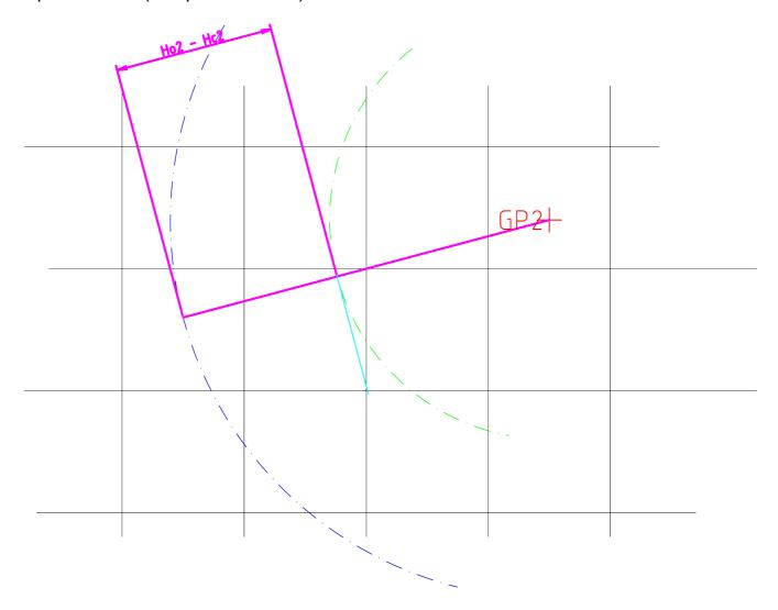
Finally, the point where the two position lines intersect is our constructed ship's position. (See picture below with in cyan CP). Note that in this example the real position (drawn in green) differs pretty much from the constructed position: this is due to the fact that both the GP's are so close to the RP and EP that the position lines are not a very good approximation anymore for the
