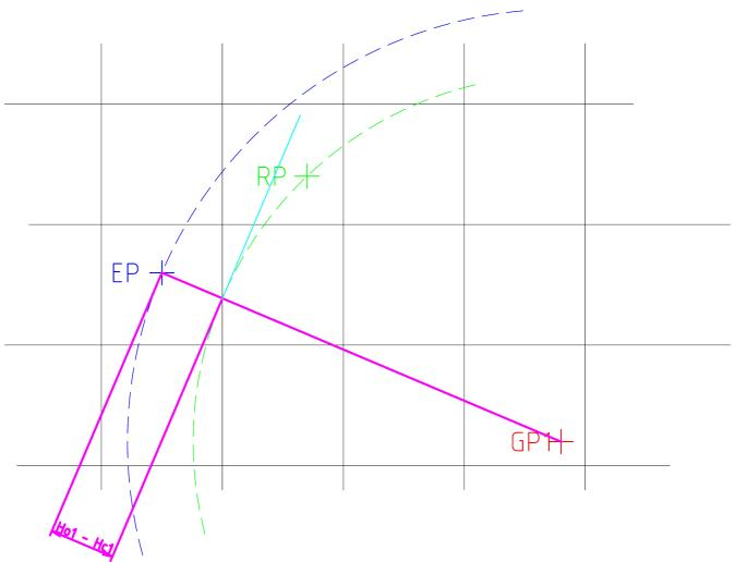
In the above picture a piece of a chart with in black: latitude/longitude grid, in blue: estimated position (EP), in green: real position (RP), and in red (ground position of celestial object 1, GP1) have been drawn.
