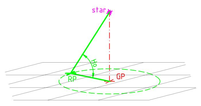
The observed altitude (Ho) of the star from the real position (RP). From all points on the green circle around GP the same altitude of Ho will be observed.
