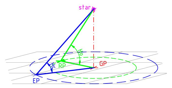
The calculated altitude (Hc) for the estimated position (EP). For all points on the blue circle around GP the same altitude of Hc will be computed. The difference between Ho and Hc in arcminutes must be subtracted from the calculated azimuth (blue line between EP and GP) in Nautical Miles to arrive at the green circle of observed altitude.
